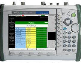
Anritsu BTS Master™ Pass/Fail screen provides status of BTS **Direct Connect Transmitter Tests**
